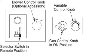
Figure 50 - Setting the Selector Switch, Gas Control Knob and Variable Control Knob for Remote Operation
